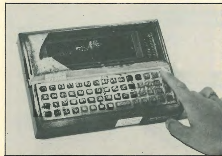
After being vandalised by burglars at the Greater London Council's welfare benefits office, this Husky Hunter computer retained all its software. The l.c. display was smashed, the main p.c. board levered out with a screwdriver, the inside sprayed with 'silver' paint, and the computer appears to have been jumped on several times. Yet its stored program and data were found to be still intact and could be downloaded through the communications port. The central processor and operating system were also found to be fully operable.
